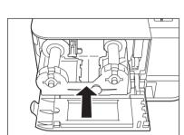
② Open the Front Cover, lift the lever and remove the sheet
