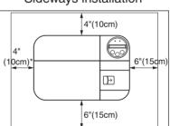
The diagram above shows the value of minimum air flow space from any walls when the Card Stacker is not
