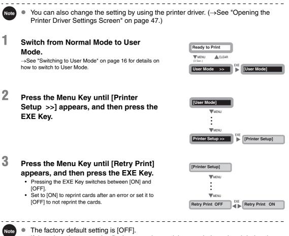
If the printer is restarted to fix the error, the card that was being printed during the error is not automatically reprinted.
