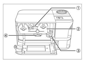
Ink Ribbon Cartridge Securing Lever Used when loading the Ink Ribbon Cartridge into the printer.
